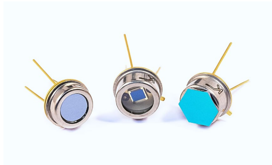
PbS and PbSe detectors with custom windows
